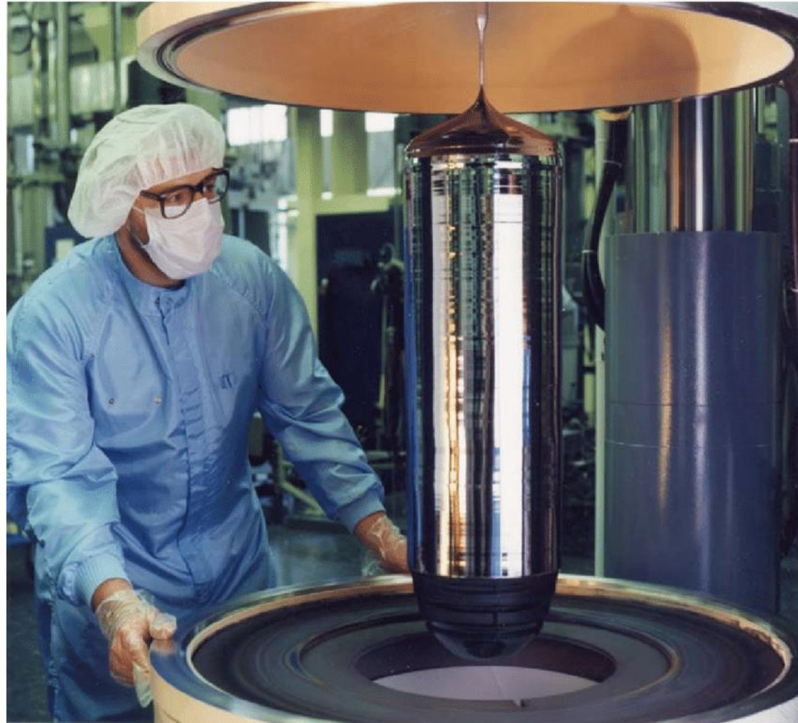
Photograph of a silicon CZ puller with 200 mm crystal
