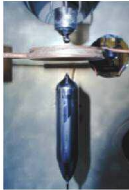
Fig. 1c. Finished FZ ingot
