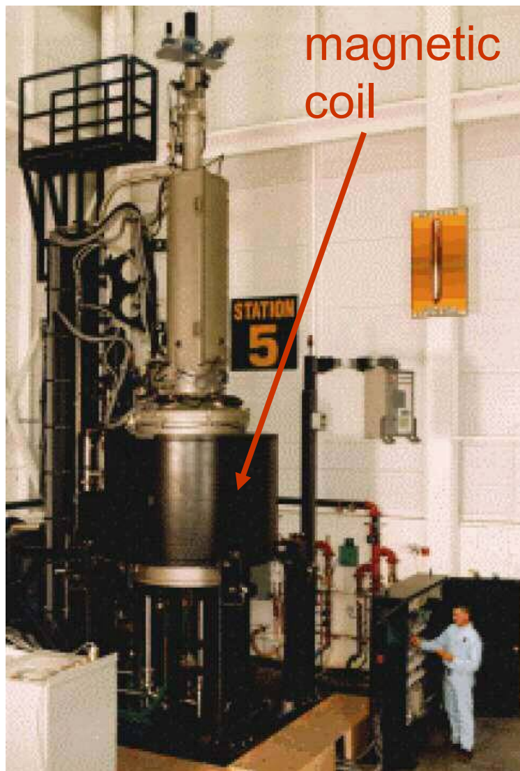
Cz. puller apparatus, Kayex company
