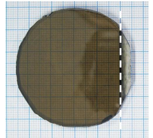
Different shape of seeds and blocking growth in lateral direction by metal borders
