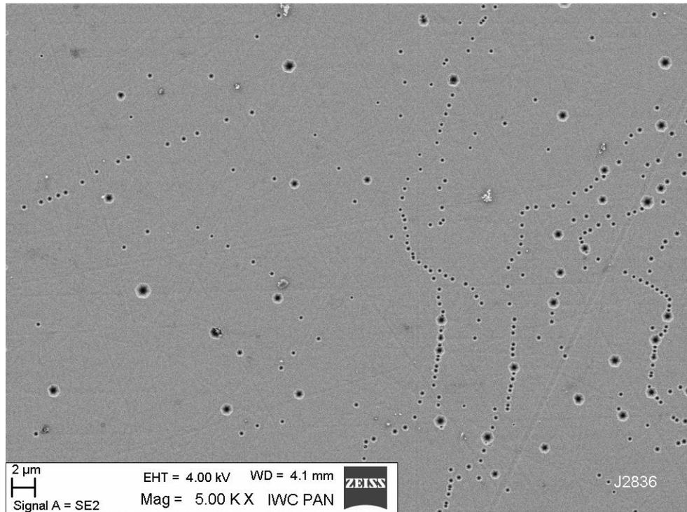
Etching performed in the liquid eutectic of KOH and NaOH at temperatures ranging from 673 to 723 K.
